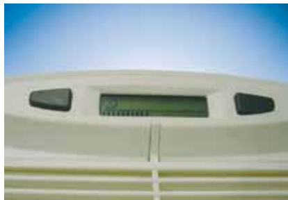
The quantity of fresh outdoor air is set with the push buttons on the top of the appliance.
